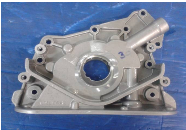
Figure 1: Front View of Oil Pump
